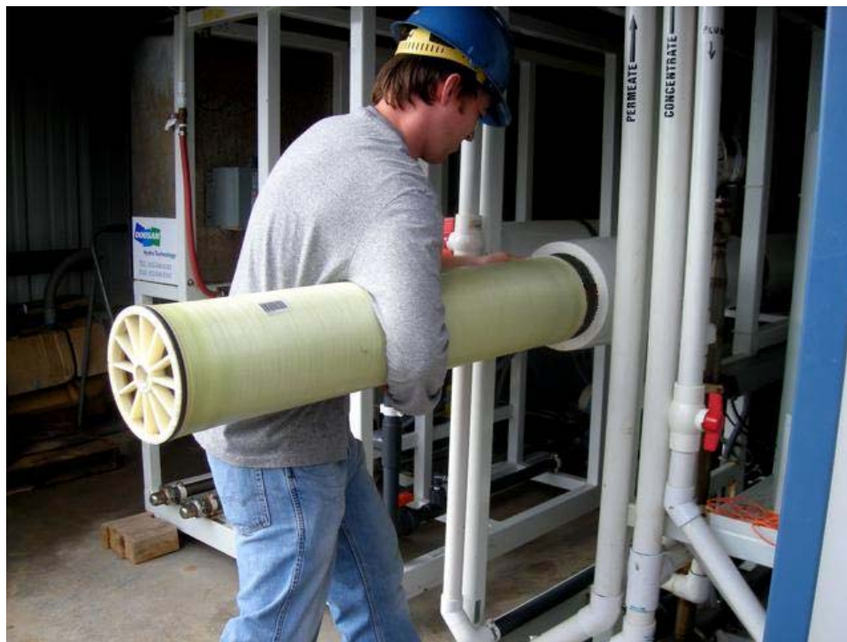
Figure ES-4: Photograph showing the loading of an RO element into the pressure vessel.
